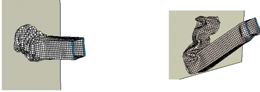
Figure 8.10: Crushing (left) and global buckling (right) of a tube subjected to impact.
